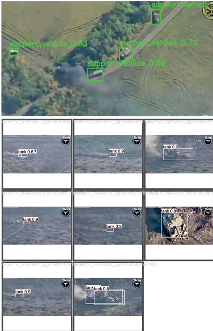
Fig. 5.14 Comparison of detection results: 1 - YOLOv8n; 2 - YOLOv11s Source: created by the authors
