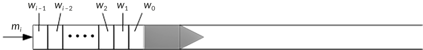
Fig. 3.5 Diagram of the formation of the incoming gas fraction at the current calculation step
