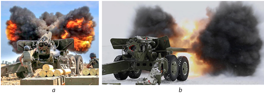
Fig. 3.3 Examples illustrating the presence of soot in the muzzle discharge: a, b – intermediate combustion phases of soot clouds recorded between the onset of ignition and full involvement of the discharge in flame
