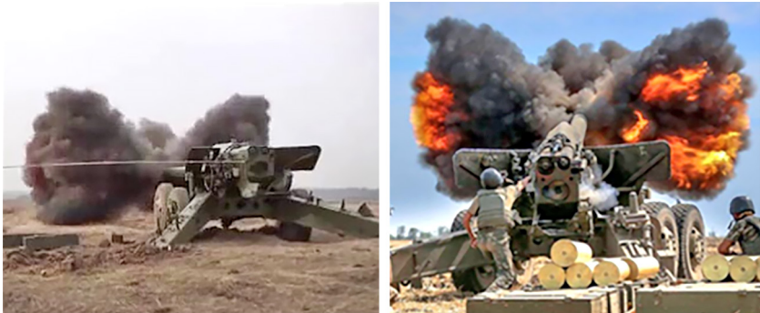
Fig. 5.8 Example of condensed carbon (soot) ejection during firing
