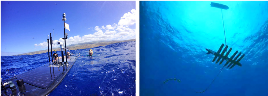
Fig. 8.4 Wave glider unmanned surface vehicle
