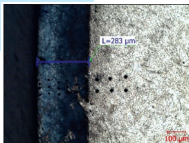
Fig. 3.39 Imprints of microhardness measurements (etched polished)
