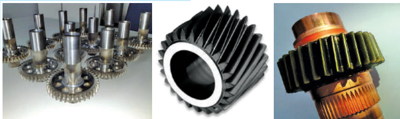
■ Fig. 4.7 Serial nitriding of gear wheels (34NiCrMoV14-5)
