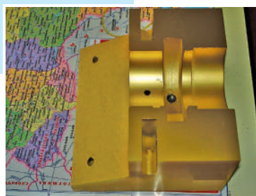
■ Fig. 3.61 Technological equipment for producing liners with Avinit hardening anti-friction coating
