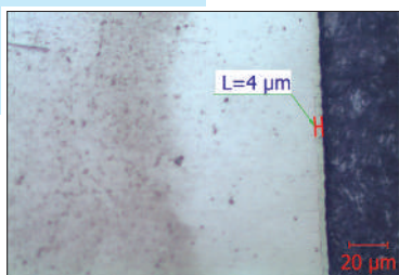
Fig. 3.45 Alphated nitrided layer from side No. 1, \times 500
