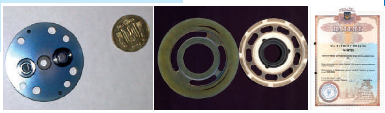
Fig. 4.5 Slide valves of hydraulic units with Avinit C 310 coating [25–28]
