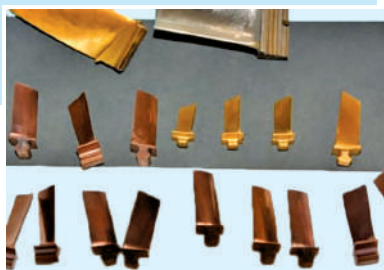
□ Fig. 3.29 Avinit C350 coating based on (Ti-Al-N)
