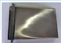
□ Fig. 3.30 Avinit D100 coating based on Ti-C
