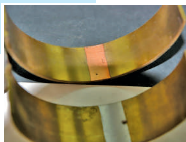
■ Fig. 3.60 Avinit anti-friction coatings on the sliding bearings (liners) work surface for internal combustion engines
