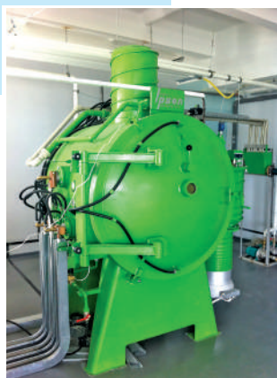
□ Fig. 4.10 One-chamber vacuum automated installation of diffusion welding and heat treatment of parts
