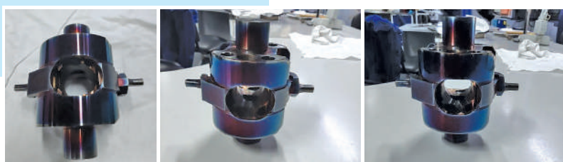
Fig. 4.3 Hydraulic units cradles with Avinit C310 nanocoating
