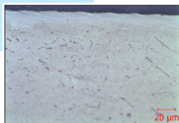
Fig. 3.46 Nitrided layer from side No. 2, \times 500
