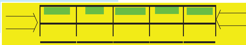
Fig. 3.64 Layer of layers of single FC with electrolyte based on barium cerates
