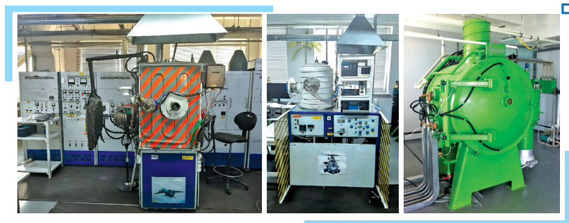
□ Fig. 2.1 Avinit vacuum-plasma automated cluster
