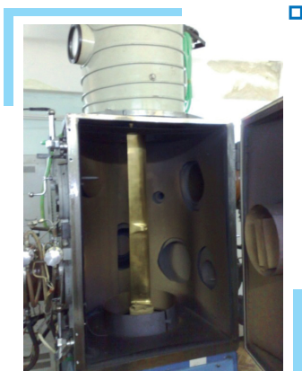
□ Fig. 4.3 Turbine blades in the course of coating deposition
