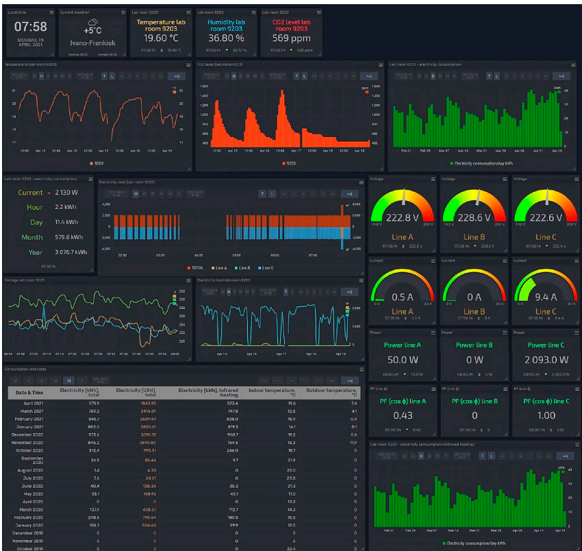
Fig. 5.9 An example of an information panel for a segment of the information and measurement system for energy monitoring in a university classroom
