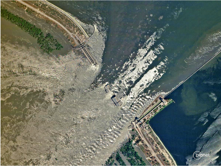
Fig. 8.2 Satellite image of the breached Kakhovka Dam Source: [19]
