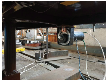
Fig. 4.14 The vibration exciter with unbalance position sensor
